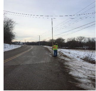
Low Clearance Overhead Utility
