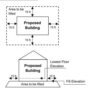
Fill must extend at least 15 feet in all directions from the proposed building. All fill within 15 feet of the building must maintain the minimum elevation noted above. Beyond 15 feet fill, fill may be tapered down to original grade or may be contained by a retaining wall.
